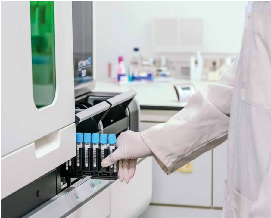
Continuous sample loading and unloading enables users to respond quickly to workload fluctuations. There is a dedicated loading position for urgent samples, as shown above.
